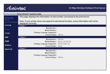
For each printer connected to the Print Server, its manufacturer, model number, supported printing languages, and current status is displayed.
